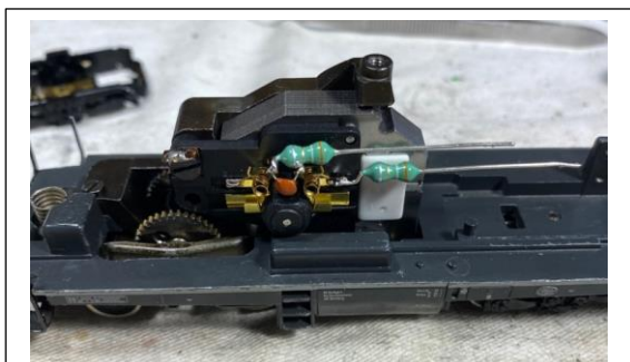
Fig. 17 – Motor upgrade complete
