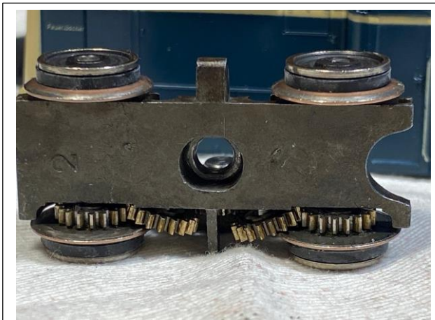
Fig. 13 - Bogie with worn gears
