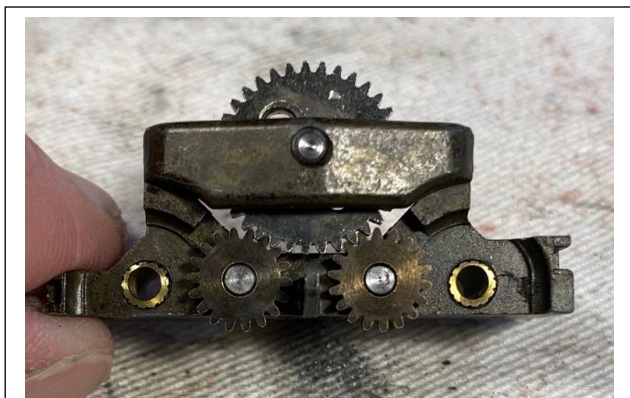
Fig. 15 – New gears installed
