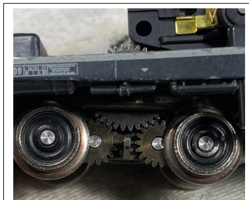
Fig. 16 – New gears installed
