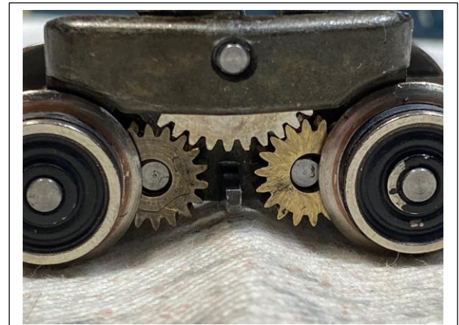
Fig. 14 – Worn gears on axles
